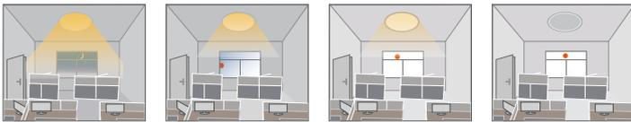
When ambient light levels fall below the set lux level, the sensor will adjust the luminaire to compensate (e.g. if ambient levels increase, the luminaire brightness will decrease).
