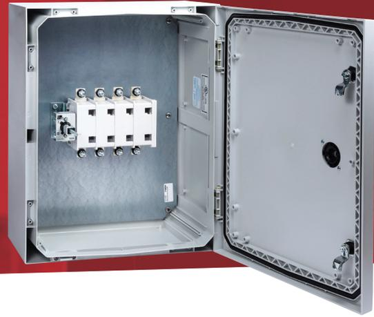
160A 4 pole switch disconnecter in a glass reinforced polycarbonate enclosure to IP65 IK10. Enclosure has separate lock and reversible door. The switch handle is padlockable and defeatable. All terminals are provided with shrouds.
