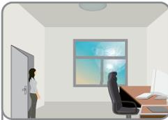
With sufficient natural light, the fitting does not switch on when presence is detected.
