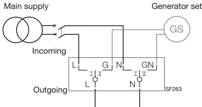
(GB) This modular changeover switch is not a disconnector. The isolation must be ensured with an appropriate device.
