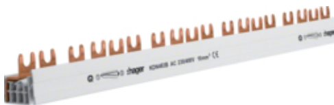
Insulated busbar 4P 63A fork 10mm 2 57M
