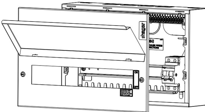
Lift door and loosen the two captive screws until the cover can be removed.
