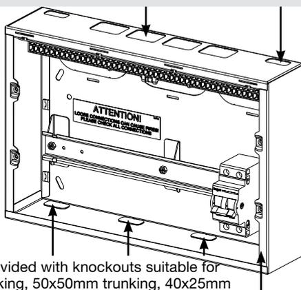
These metal units are provided with knockouts suitable for use with 100x50mm trunking, 50x50mm trunking, 40x25mm trunking and also large rear knockouts. Grommet strip is provide to protect the cables when entering the board.
