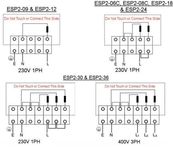
4.1 Follow the above diagrams making sure you use the correct diagram for the model you are wiring. Incorrect wiring may damage the unit and is not covered by the guarantee.
