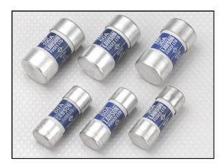
Lawson Type "ME" and "MF" fuse-links are for use in single or three-phase house service cut-outs or similar installations. The standardized BS 1361 breaking capacity of these fuse-links is 33kA at 0.3p.f. However to cater for increasing fault levels all Lawson house service cut-out fuse-links have been ASTA tested to 80kA at 0.15 p.f.
