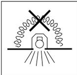
Ensure free movement of air around the fitting by removing any roof void insulation from at least 140mm around the hole.
