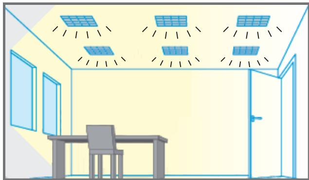
**EN** If the preset configuration is for Presence detection, making a movement should turn the lights on. If the preset is for Absence, turn the light on at the switch and carry out the following additional steps...
