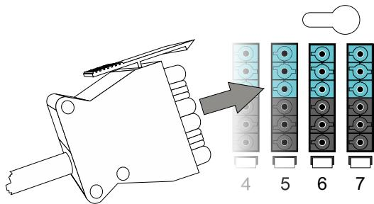
**EN** Plug the luminaires into the LCM.
