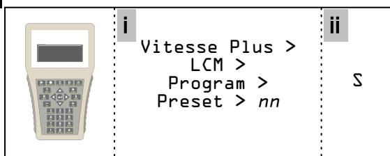
**EN** Use the UNLCDHS handset to send the required preset configuration to the LCM.
