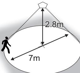
**EN** This device is designed to be ceiling-mounted.
