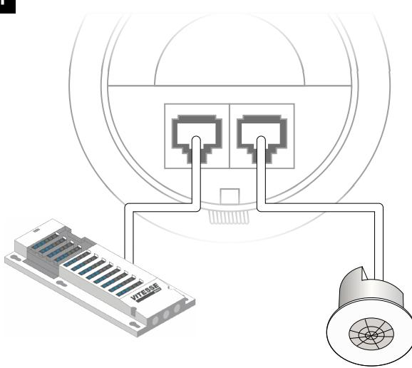
**EN** Use the two RJ45 sockets with Cat5 patch leads to connect other Vitesse Plus components such as lighting control modules (LCMs) and detectors.
