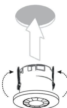
**EN** Bend the springs up and push detector through hole in ceiling. When fully inserted the springs snap back to hold the device in place.
