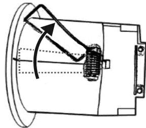
**EN** Remove or bend both springs so that they do not stick out over the sensor head bezel.
