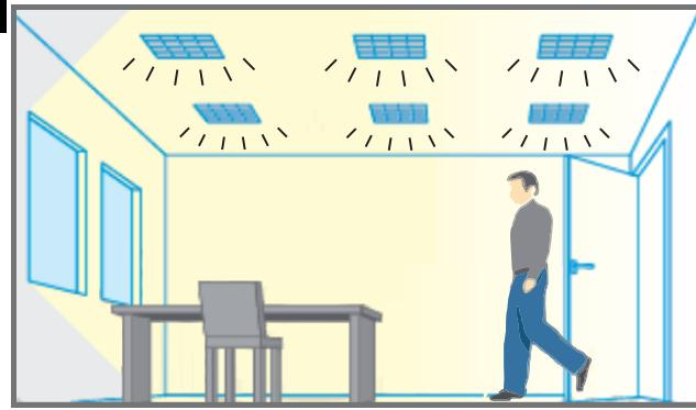
**EN** Enter the room and check that the load switches on.
