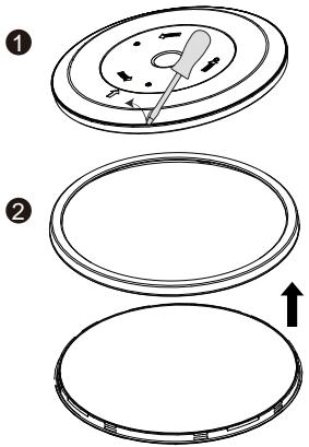
1. Remove the diffuser and light guide plate.
