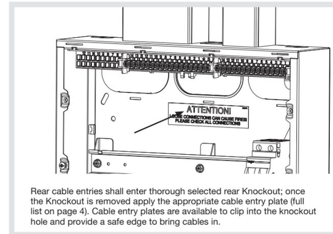
Rear cable entries shall enter through selected rear Knockout; once the Knockout is removed apply the appropriate cable entry plate (full list on page 4). Cable entry plates are available to clip into the knockout hole and provide a safe edge to bring cables in.
