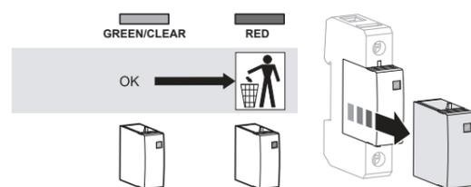
Where surge protective devices (SPDs) or other equipment are likely to influence the verification test, or be damaged, such equipment shall be disconnected before carrying out the insulation resistance test.
