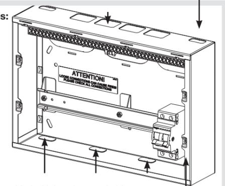
These metal units are provided with knockouts suitable for use with 100x50mm trunking, 50x50mm trunking and also large rear knockouts.
