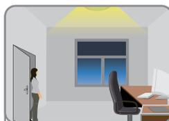
With insufficient natural light, the sensor switches on automatically when someone enters the room.
