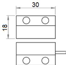
Parameters of relay reed switchboard
