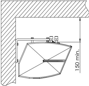
**Wall installation by means of a horizontal bracket**
