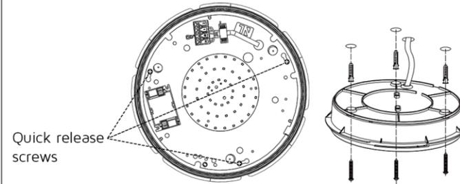
**Step 3:** Wire the Gear Tray as per the diagram below.
