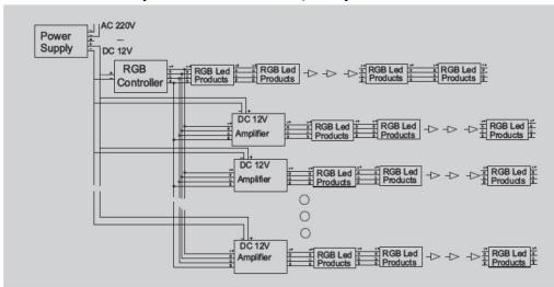
structure four: parallel connection, two or more power switch.
